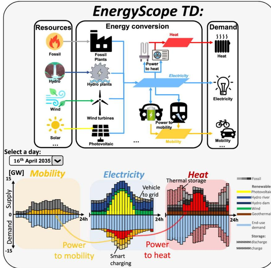
Figure 7: Overview of an energy system in Energyscope.
