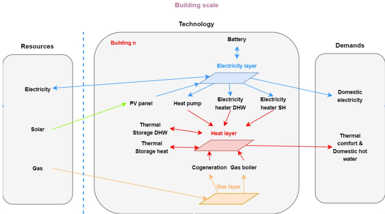
Figure 4: Predefined Energy System Model at Building Scale in the Renewable Energy Hub Optimizer (REHO)
