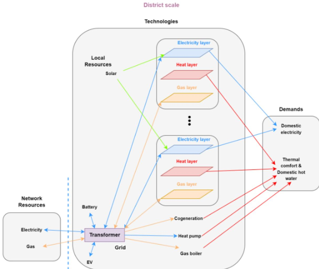
Figure 34: Predefined Energy System Model at District Scale in the Renewable Energy Hub Optimizer (REHO)
